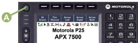
After a short time, the red, yellow and green LEDs light up. The display then shows Zone and channel text, and menu items display on the screen.
